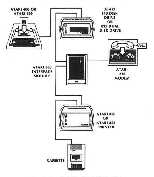
Figure 1 Using the ATARI 820 or ATARI 822 Printer
