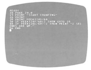
The next program turns on your Program Recorder and allows it to run for 4 seconds. The Program Recorder turns off automatically.
