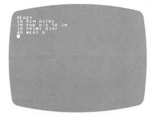
When setting up an array it is necessary to store values in each variable in the array, as in the following example. Run the next program, and then check what is in each variable with a **PRINT** instruction, such as **PRINT** A(3).
