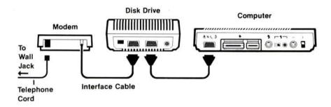
3. Plug one end of the telephone cord into the phone jack on the back of your XM301 Modem and the other end into a telephone wall jack.
